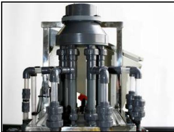
This is a new proportional injector for agricultural fertilizers with a new design. With this we reduce a 70% of volume (very interesting for transport costs), we also reduce the power of pump, but chiefly this equipment works hydraulically better over previous, keeping the same pressure in every injector.
